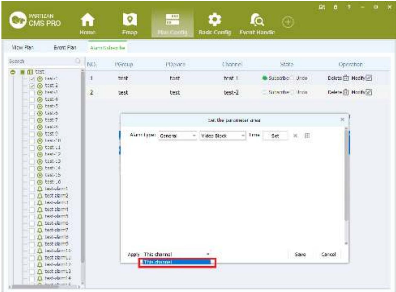
Figure 8-18 Setting protection channel
